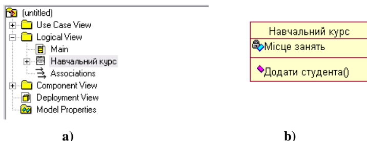
Fig. II.2.13. a) A class created in a browser window b) Notation of the UML language for the class
