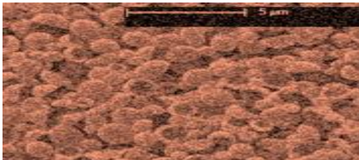
Fig.1. SEM images for turmeric from aqueous solution, retained on the cellulose/elastin membrane with plasticizer and gemini surfactant: polymethylene- \alpha , \omega -bis (N, N-dialkyl-N-deoxy-d-glucitolammonium iodides)
