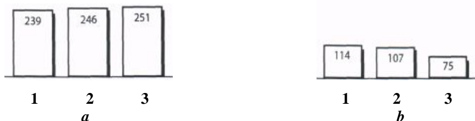
Fig. 2. Distribution of equivalent stresses in the wheel toothed \sigma_{ек} (a) and the shaft \sigma_{еВ} (b)
