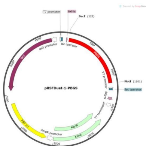
Figure 3.6 Schematic diagram of the pRSFDuet-1-PBGS expression vector
