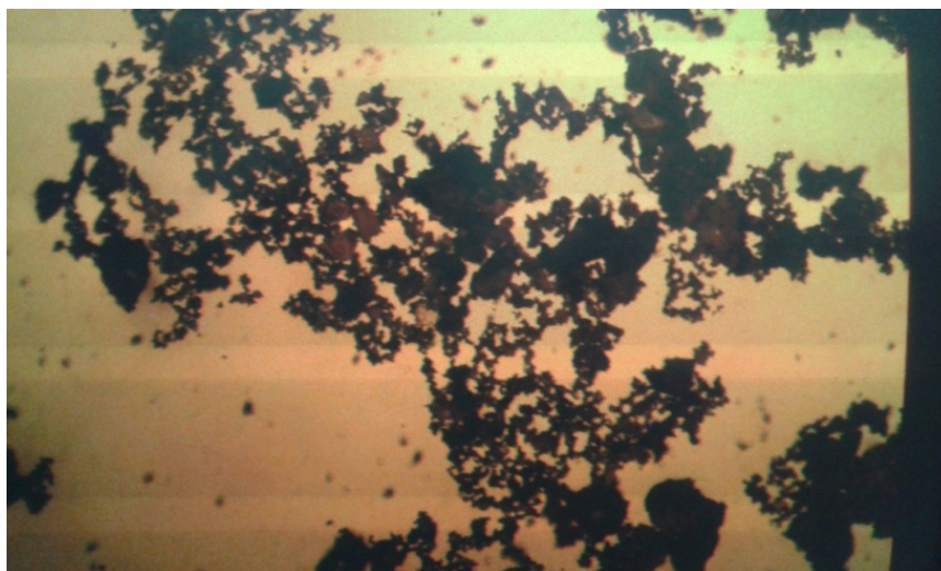
Fig 1. Micro particles of manganese dioxide obtained from fluorine – contained electrolyte at the magnification x 600
